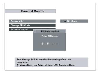
The age rating control, the PIN(Personal Identification Number) Code and the passwords to various menus can be configured. The PIN Code box will automatically appear when this menu is selected. The default PIN Code is 0000.
